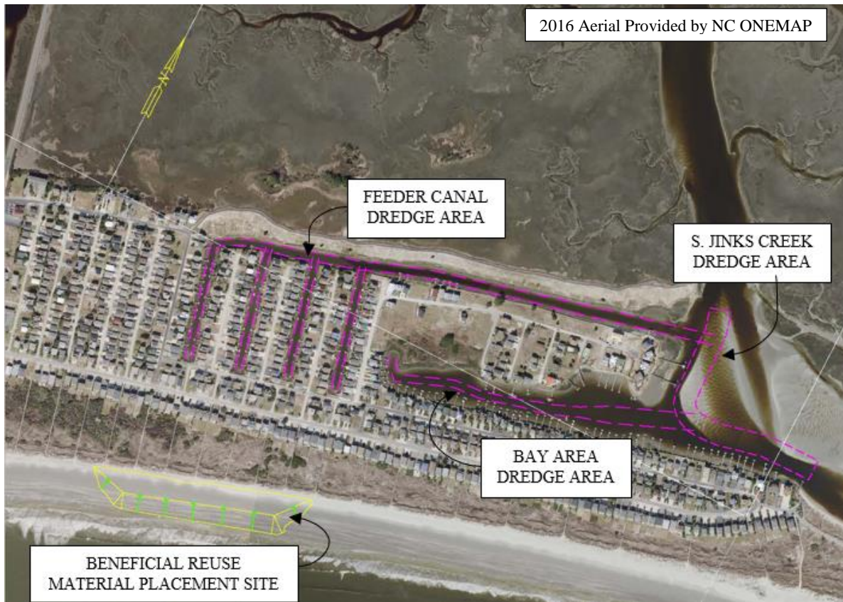
Figure 4. South Jinks Creek, the Bay Area, and Feeder Channel Work Areas
