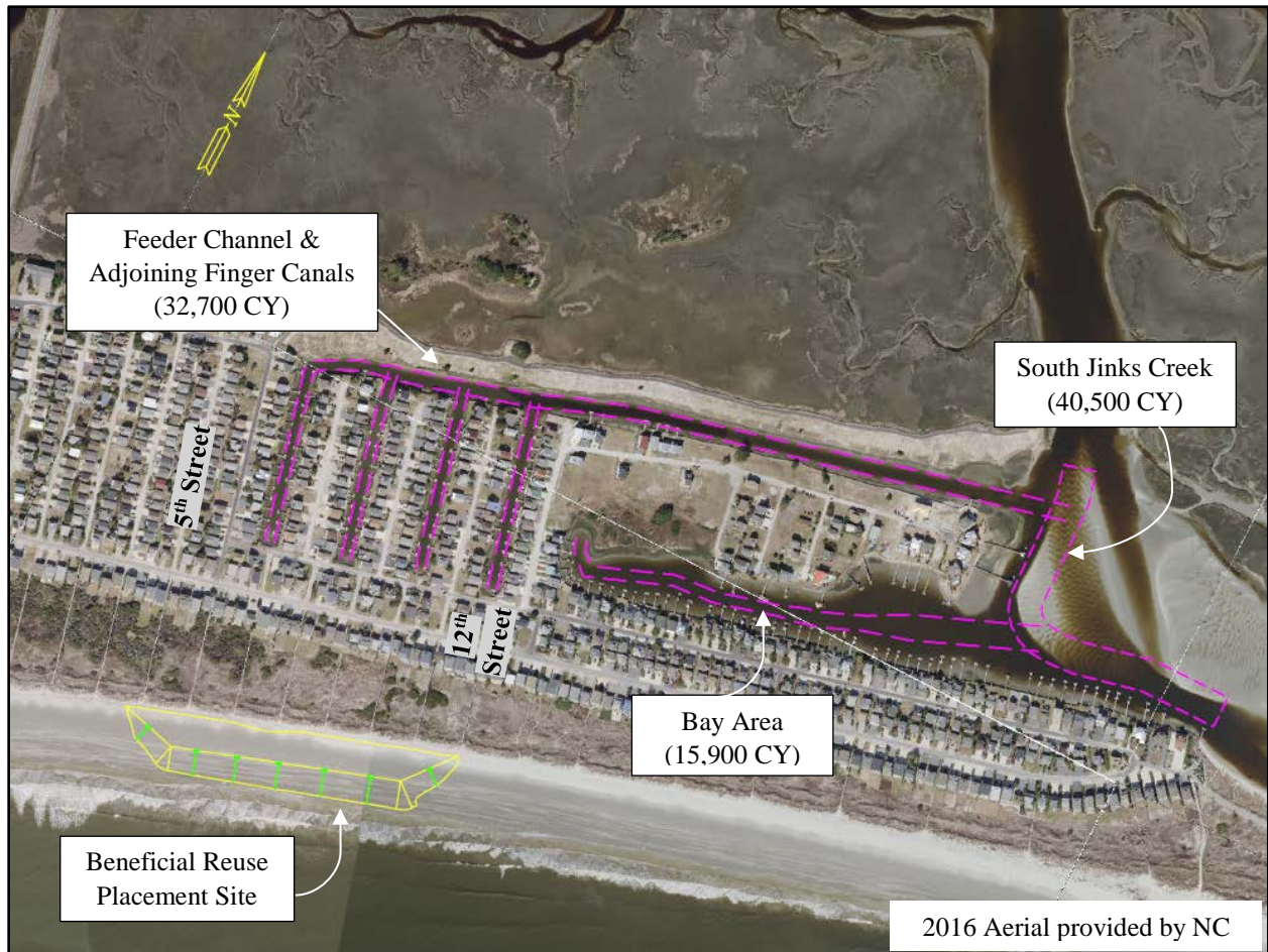
Figure 2. South Jinks Creek, the Bay Area, and Feeder Channel Work Areas
